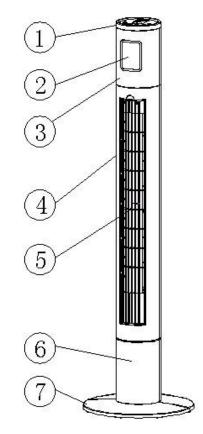
CAUTION: THIS FAN MUST OPERATE IN THE UPRIGHT POSITION ONLY. DO NOT LAY FAN ON ITS SIDE OR IN ANY OTHER POSITION. DOING SO MAY CAUSE DAMAGE TO THE FAN AND/OR PERSONAL PROPERTY. DO NOT USE THIS FAN WITHOUT ITS BASE.
