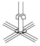
Retighten the height adjustment ring to prevent slipping, then place the fan assembly onto the pole and tighten the pole screw manually.
