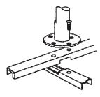
Loosen the height adjustment ring and extend the support pole to your desired height.
